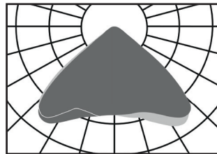
Variant 3: PrimeLine 03 Light distribution: symmetrical 105°
