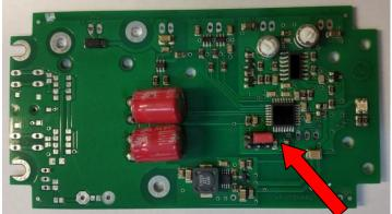
After connecting or disconnecting the jumper, the device must be restarted.
