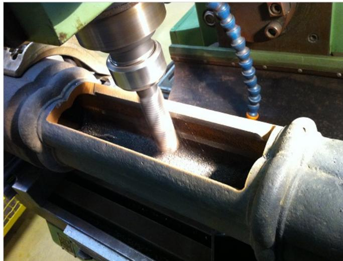
*Milling work on the mast for a flap access panel*
