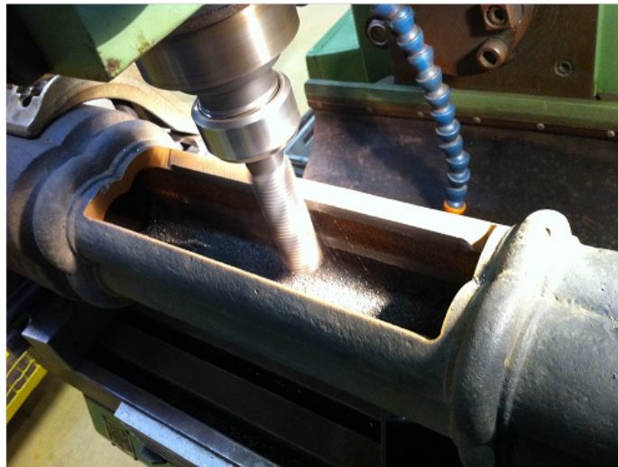
Milling work on the mast for a flap access panel
