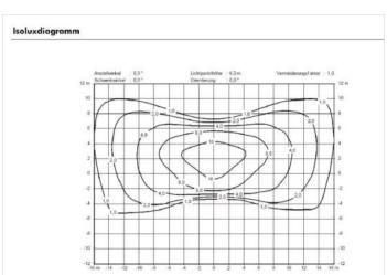
Above and below: Light intensity distribution and ISOLUXDIAGRAMM for ME618
